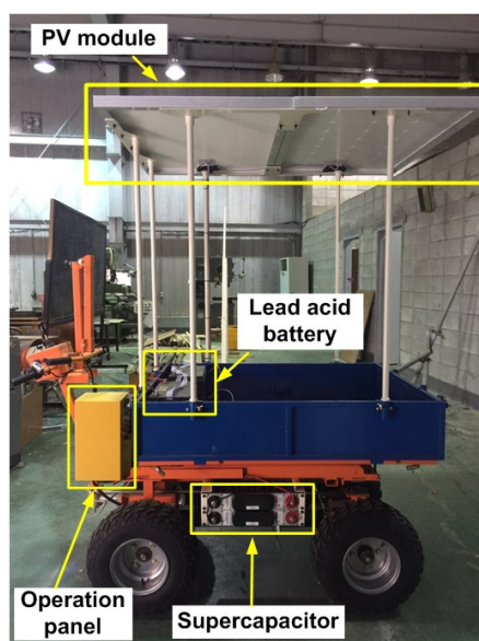
Figure 1. Configuration of electric carrier used in this study
