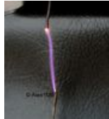
555 timer based plasma speaker by Alex1M6
