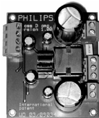
Gambar 2. Evaluation Board Philips UcD UM10155, 200W 4 ohm
